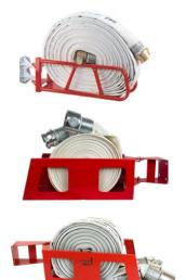
SRI hose cradle is the free swing type with 180° movement suitable for holding one length of 2½" x 30 m layflat fire hose. It is installed next to the wet or dry riser outlet.
